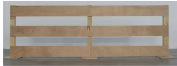
Figure 3: View of fall protection guardrail mock-up developed and used for this study.
