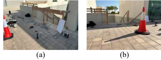
Figure 6: (a) View of the scenario where the mock-up misses the mid and toe boards and has clutter on the floor, and (b) same condition with only vertical poles installed.
