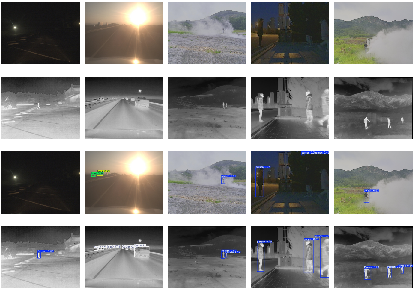
Fig. 6. Detections on low visibility conditions. First and second rows: RGB and corresponding IR images. Third row: YOLO detections on the RGB images. Notice missed and wrong detections in the visible range. Forth row: Detections on the IR images using the trained network over the automatically labeled dataset.
