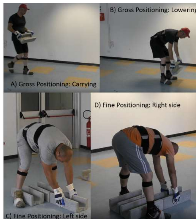
Figure 6. Images showing (A,B) carrying and lowering the cable duct during the “gross” positioning task and (C,D) the “fine” positioning of the cable duct on the left and right sides.
