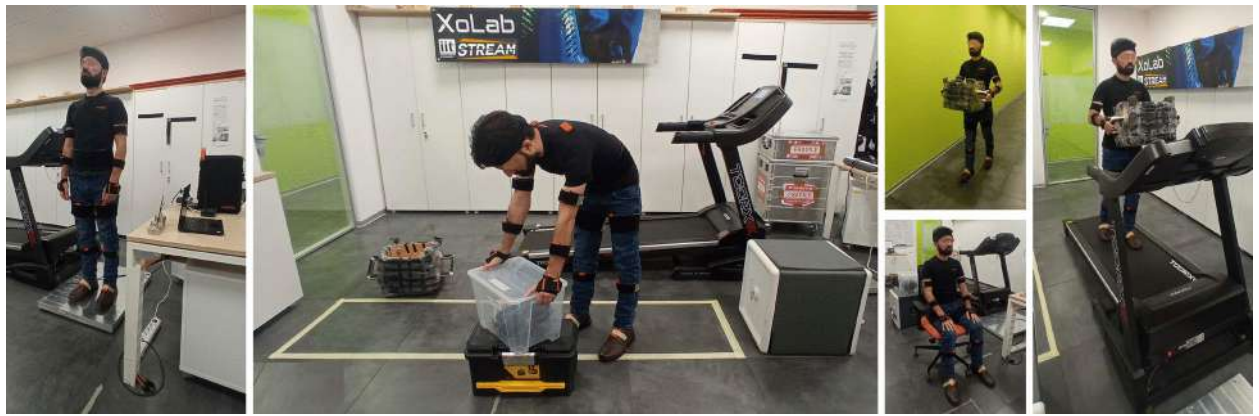
Fig. 1. The figure shows on the left how the sensors were worn by the test subjects. In the centre there is an image of the subject performing an asymmetric stoop and the rectangle defining the lifting activities area. This also shows the position of the stations according to the rules in Section "Experimental protocol". The right side of the picture shows the worker while carrying a load (flat surface), sitting, or carrying a load on an inclined surface.
