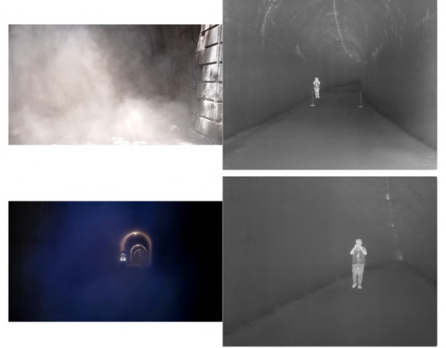
Fig. 5. Comparison between RGB camera (left) and IR camera (right) in challenging situations. Note that the aspect ratio of the images vary (4:3 for IR and 16:9 for RGB)
