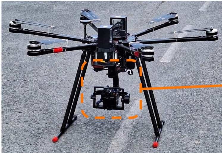
CATEC C750 Drone with Road Maintenance Payload
