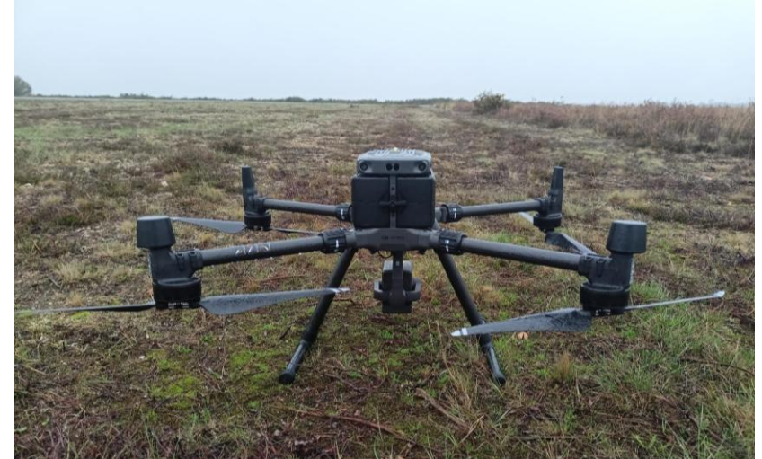
DJI M300 Drone prepared to perform road construction photogrammetry
