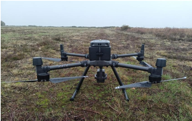
DJI M300 Aerial Robot with Zenmuse L1 Payload
