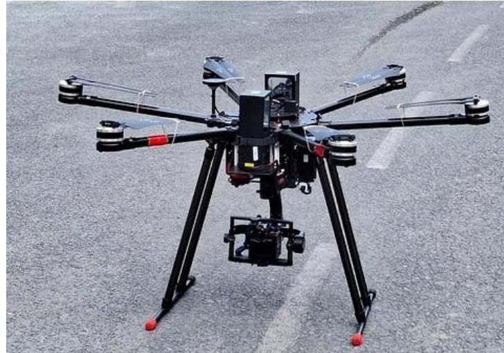
C750 Drone prepared to perform autonomous road maintenance tasks
