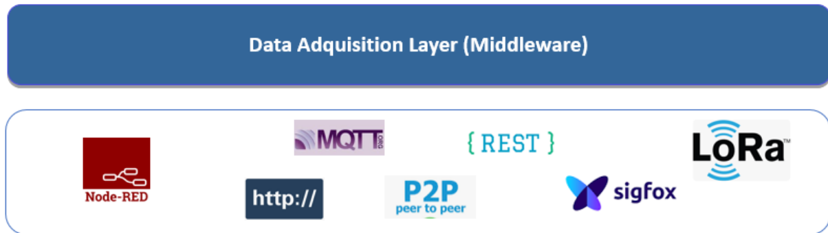
Figure 27. Digital Twin Data Acquisition Layer
