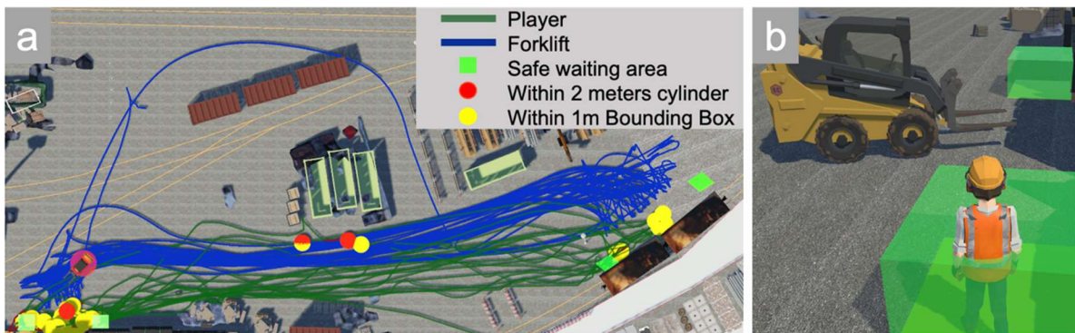
Figure 21: (a) the results from training scenario 2 indicating the trajectories and proximity events, and (b) the safe area where the trainee can wait for the forklift.
