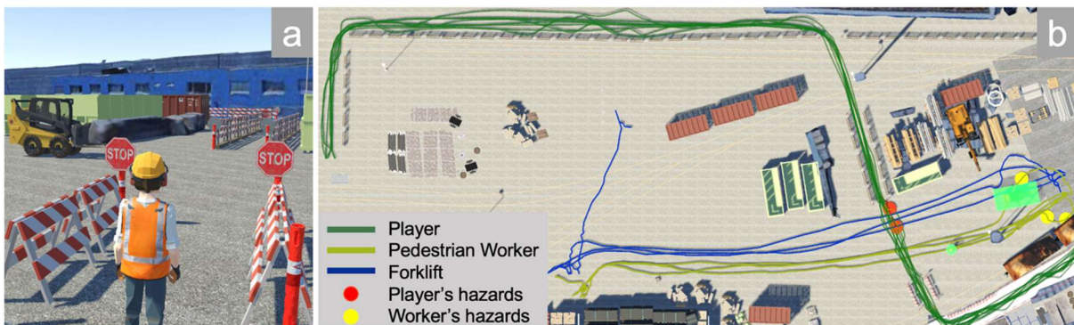
Figure 20: (a) Results of the first training scene, incl. the landscape, BIM model, resources, and trajectories from IoT devices, and (b) the trainee crossing the road while the forklift follows the real-world trajectory.
