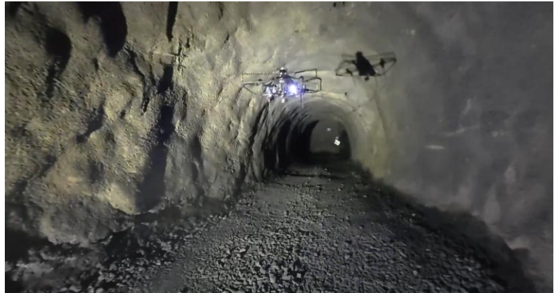
CADRIN Drone performing autonomous flight inside tunnel
