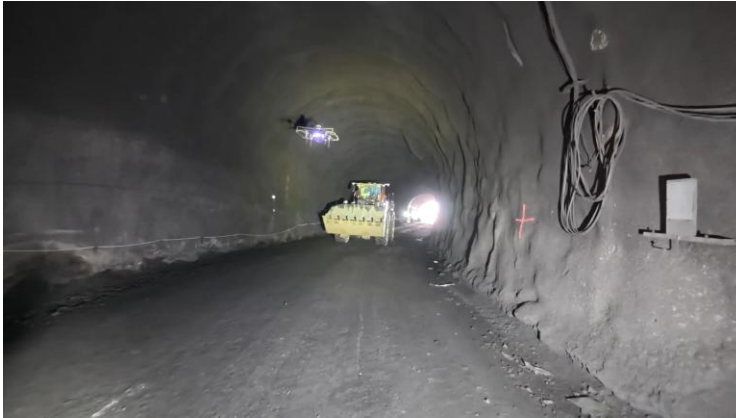
Aerial Robot and Autonomous Wheel Loader cooperation inside of the tunnel (Left: Real video recorded on-site; Right: Drone's sensor view)
