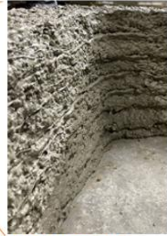
Printed structure for mechanical performance tests
