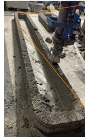
Printed structure for mechanical performance tests
